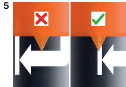
To unlock syringe fully rotate
