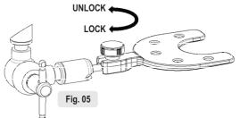
**05- Dentulous bitefork (12):** Position the bitefork in the transfer set until the transfer set limit and use the screw to fix it (fig.05).
