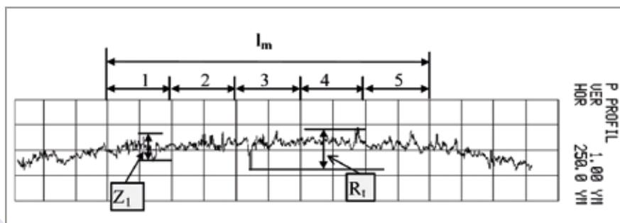
Fig. 2: A surface roughness of more than 1 µm remains in titanium even in case of optimal treatment<sup>[2]</sup>
