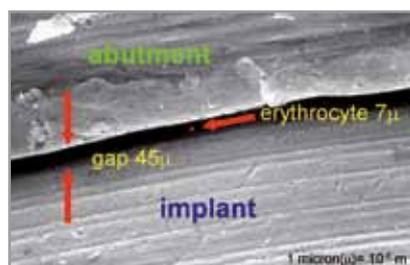
Fig. 3: Size of an erythrocyte and implant-abutment-gap relation (magnification 1:750).
