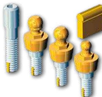
This component is manufactured from bio-compatible materials with an "elastic" memory. While screwing in the attachment, the insert is compressed. When the threaded attachment is fully seated, the elastic insert will expand and return to its original form, which prevents rotation and unscrewing of the device. The insert is applied at the manufacturing facility UPON REQUEST. It can be applied to any screw with a diameter greater than 1.8 mm.
