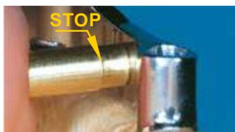
Insert the housing shaper into the hole and lock it in place using resin. Be sure not to go past the "STOP" when applying resin
