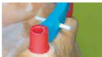
Model the bar in resin and drill a 0.8 mm hole in the most ideal position. Insert the ceramic pin through the hole.
