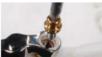
Insertion of the Ot Equator seeger inside the self-extracting peek ring already in position.
