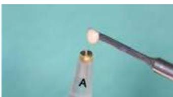
Place a small amount of two-part self curing "metal to metal" resin inside the sphere.
