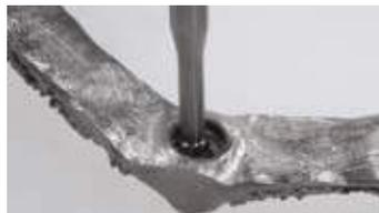
Special cutter used to clean off oxide or any small bubbles inside the cast core.
