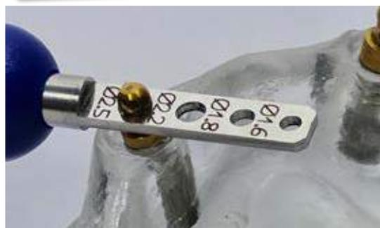
Rhein83, always aware of the needs of dentists and dental technicians, created a very simple but essential tool. The sphere measuring gauge provides an easy and safe way to check the diameter of spherical attachments through his four holes corresponding to the most common sizes: 1.6-1.8-2.2-2.5mm.
